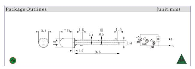
Remark:1. All dimensions are in millimeters, tolerance is 0.25mm unless otherwise noted.
